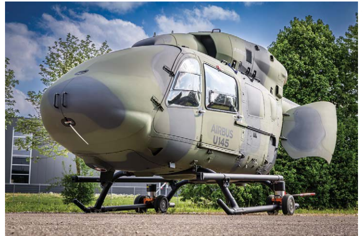
The U145 combines the proven airframe, power and useful load of the H145 with the autonomy of a UAS.
