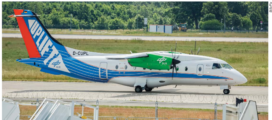
A Dornier 328-100 is being displayed outside Hall C (pictured). The aircraft has been converted into a flying testbed for climate-friendly air transport technologies as part of the UpLift project. It will be used to measure and
