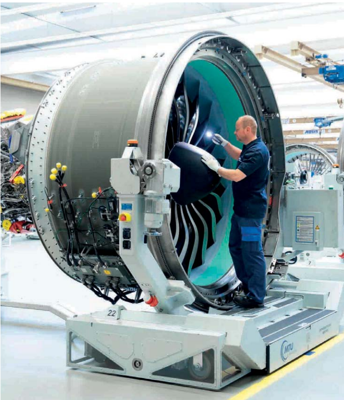
Technician works on a Pratt & Whitney PW1100G engine at MTU's Munich headquarters.
